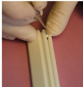
Drawing the instrument through the Narrow Honing Channel<sup>®</sup> White Clearance<sup>™</sup> Stone during the sharpening stroke
